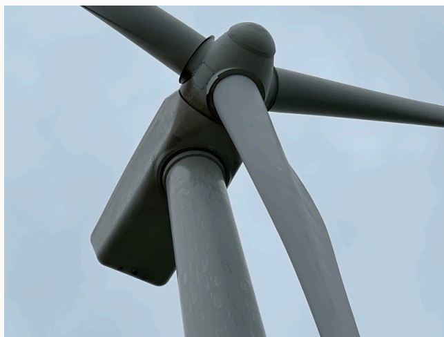
Grease leak from a blade bearing in the UK without ground pollution:
